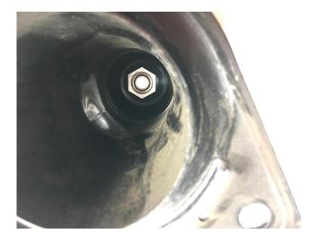
Step 3. Using a 32mm Socket on the Carrier & Nut Torque to 45 foot pounds
