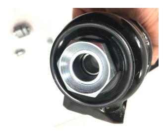
Step 4. Reassemble your suspension & Remove Any Wide Steel Spacers Previously Intended as a retainer for the original Rubber Bushings.
