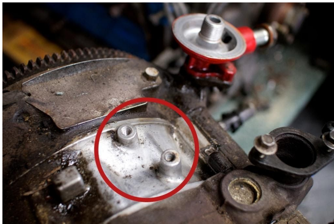
Image 3: Recommended engine grounding location
