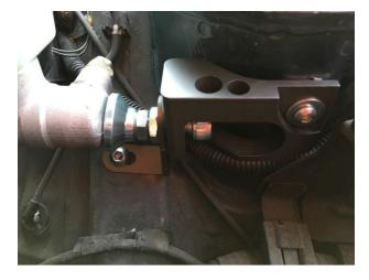
• Next adjust the main bolt length so the stopper just touches the master cylinder face. To adjust the height of the stopper up/down or left/right, grab the main billet bracket and move it into position. Once the assembly has been positioned correctly, tighten down the M6 and M8 nuts.
