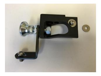
Use a Ball-End Allen Key to move the main bolt into position if it is difficult to spin by hand. You
