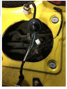
Next you will de-pin the fuel pump connector. If you have never done this you can check out our video on connector de-pinning on our youtube channel. This is not the same exact connector as in the video, but they are both Sumitomo connectors so the de-pin process is the same. Before you de-pin the connector take note of the position and color of each wire, this will be important later.
