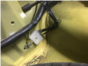
Now the last step, take the long, red power cable and run it to your battery. There are many popular battery locations on an FD, so we have made the power wire able to be cut to length. Just snip the fuse off the wire, run it through the car as you prefer, and use the provided heat shrink type butt connector to connect the wire to your positive battery terminal after trimming the wire to length.
