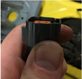
Now, BEFORE you pin the stock fuel pump connector on to our harness do yourself a favor and put the boot over the end of the harness. It is possible to work the boot over the connector, but it is quite difficult and we would not suggest it. Now you can pin the stock connector on to the new harness as shown.
