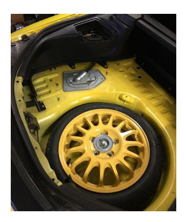
Next remove the silver fuel pump cover and disconnect the two electrical connections to the fuel pump. One of these is the 4-pin fuel pump power, ground and fuel level sensor wires and the other is the fuel pump hanger ground. Both of these connectors have tabs that must be depressed to remove
