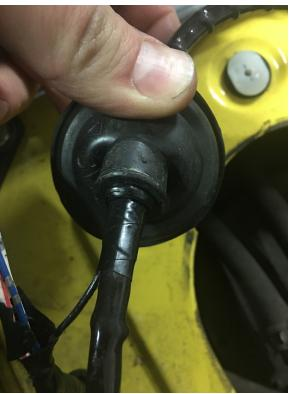
Once you have the grommet in place secure it by taping it just like stock and feed your new fuel pump wiring and your old pump hanger ground through the fuel pump cover. Work the grommet back in to place, plug in your fuel pump and hanger ground and re-install your fuel pump cover. At this point your trunk should look something like this.
