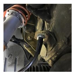
• Disconnect the soft line from the hard line nearest the chassis, and quickly wrap the hard line to absorb brake fluid which will drain out.
