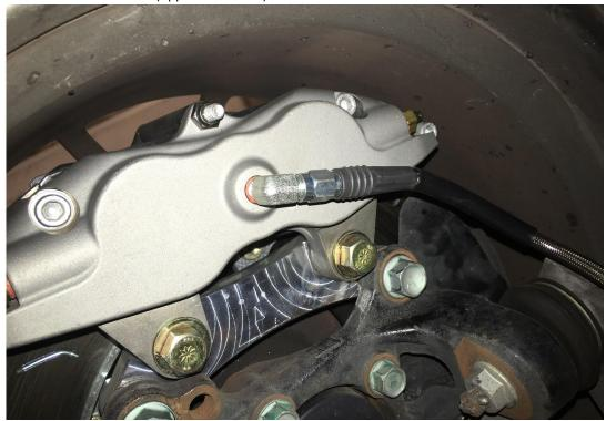
This bracket will remain fixed to the vehicle. Instead the caliper will be removed from the bracket for future servicing and pad changes.
